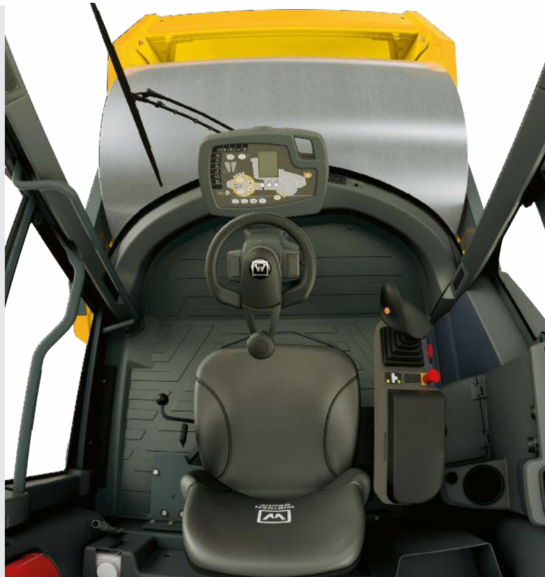
The important buttons are visible at all times in the spacious Easy Drive operator's platform. The idea behind all other operating elements is that, the more often they are used, the closer to the joystick they are located.
