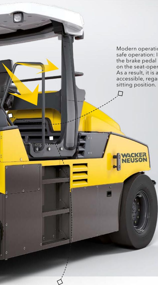
Modern operation - safe operation: In the RR280, the brake pedal is located on the seat-operating unit. As a result, it is always easily accessible, regardless of the sitting position.
