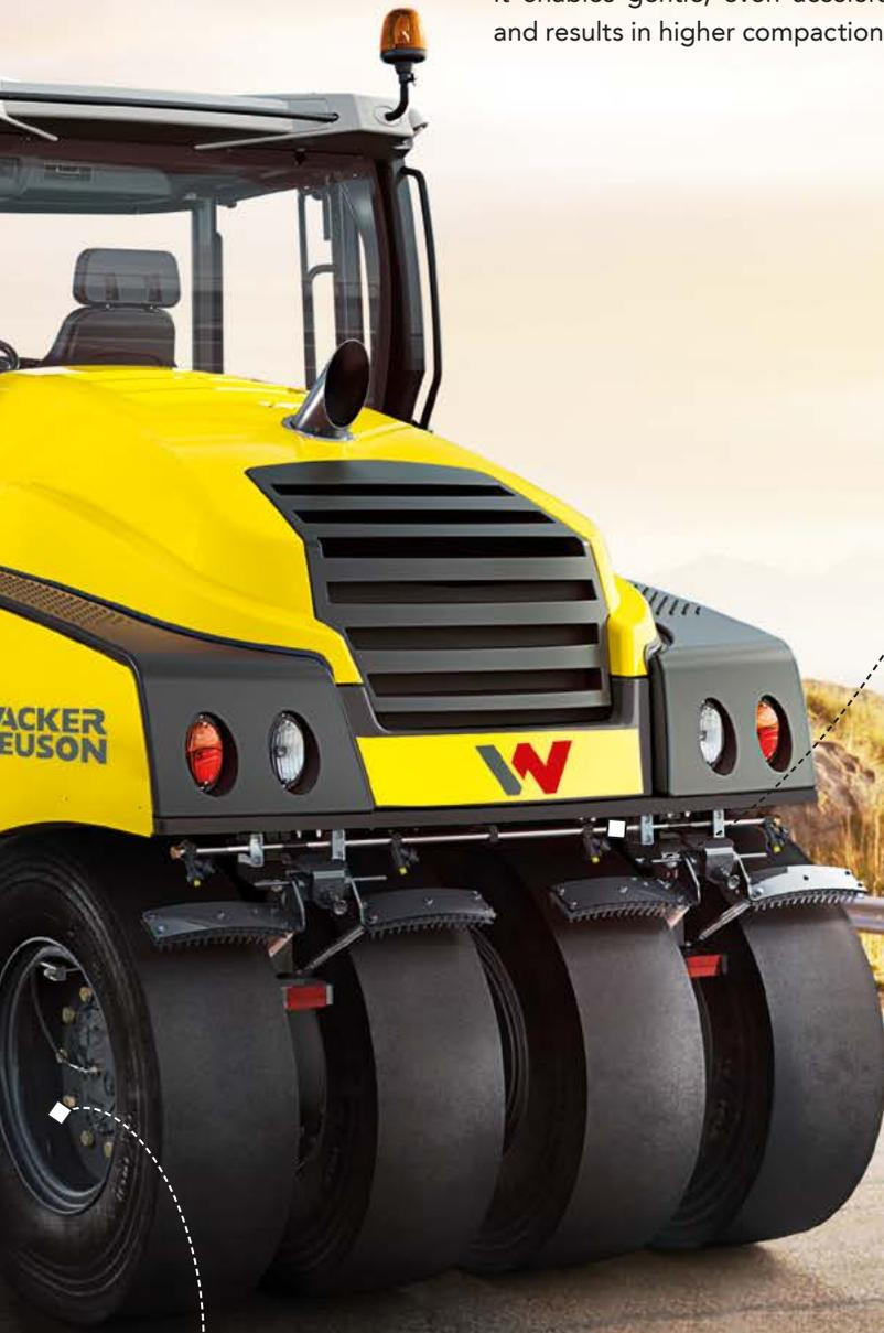
Using the tyre inflation system, the tyre pressure can be varied from 4 to 8 bar to adjust the footprint.
