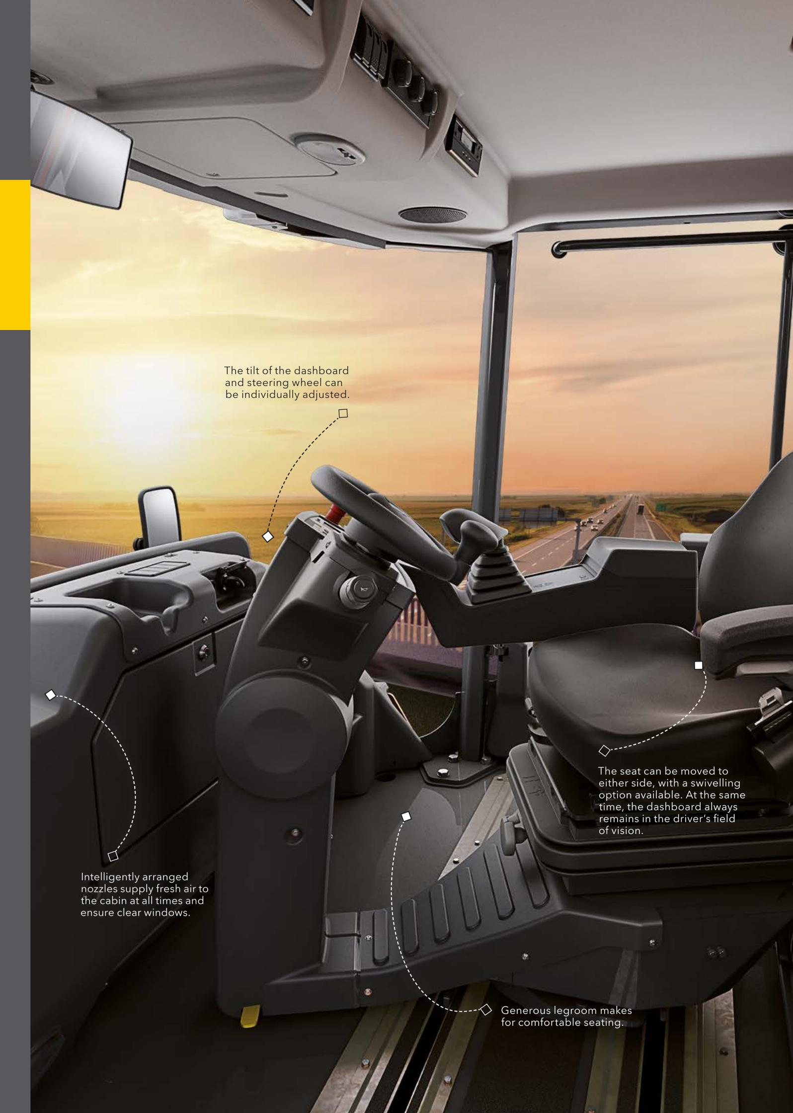
The tilt of the dashboard and steering wheel can be individually adjusted.
