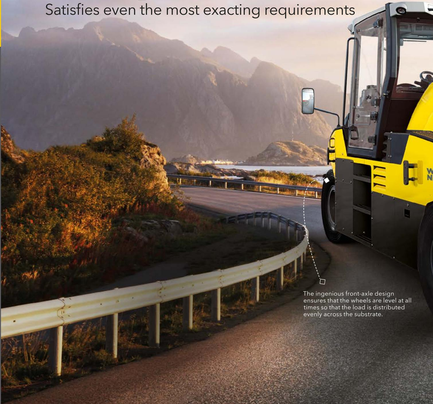
The ingenious front-axle design ensures that the wheels are level at all times so that the load is distributed evenly across the substrate.
